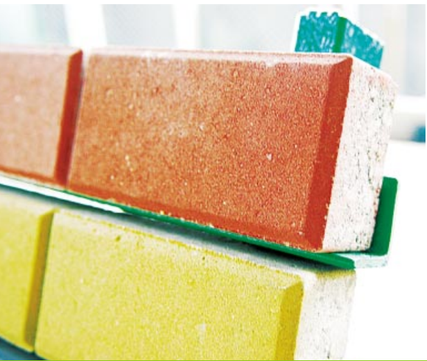
大欖懲教所預製混凝土工場利用循環再造的混合物料製成地磚。 The kerbstone workshop in Tai Tam Correctional Institution using recycled aggregates as a component to make paving blocks.
