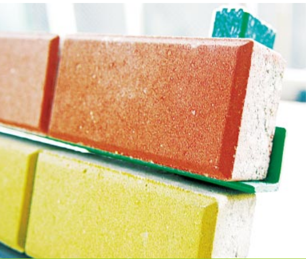
大榄惩教所预制混凝土工场利用循环再造的混合物料制成地砖。 The kerbstone workshop in Tai Tam Correctional Institution using recycled aggregates as a component to make paving blocks.
