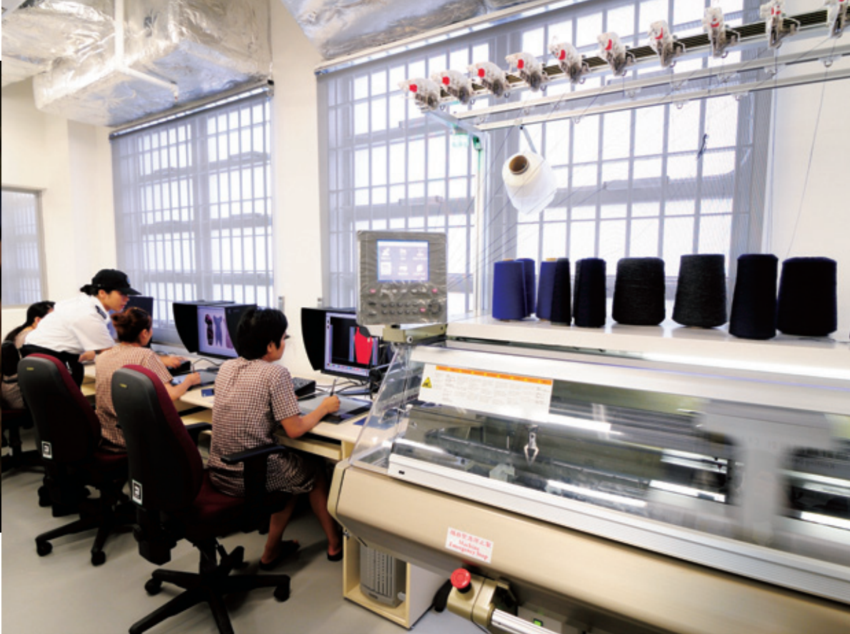
罗湖惩教所针织工场设有电脑横织机及设计系统，藉以提升生产效率，并提供市场导向的训练。 The computerised flat-knitting machine and its design workstations at the knitting workshop of Lo Wu Correctional Institution help increase productivity while providing market-oriented training to inmates.
